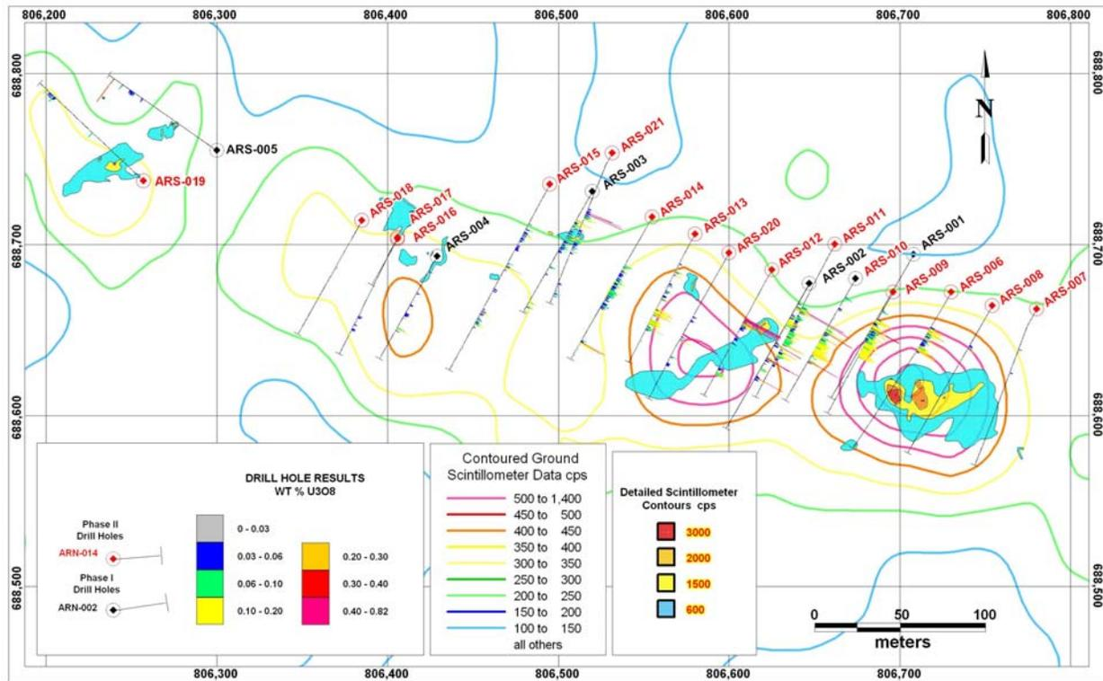
**Figure 1. Map showing the ground scintillometer radiometric anomaly at Aricheng South with the location of Phase I drill holes labelled in black and Phase II drill holes, results of which are reported here, labelled in red.**
