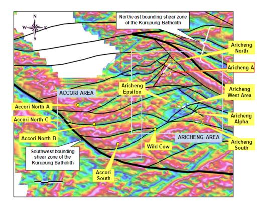
Map of airborne magnetic data from the Kurupung Batholith overlain with interpreted structures (black lines) that extend between the bounding shear zones of the batholith. Cool colours represent rocks with little magnetism while warm colours represent magnetic rocks. White irregular areas outline the footprints of uranium mineralization drilled by U3O8 Corp. at Aricheng North, Aricheng A, Aricheng Epsilon, Aricheng West, Aricheng Alpha, Aricheng South and Accori North C.
