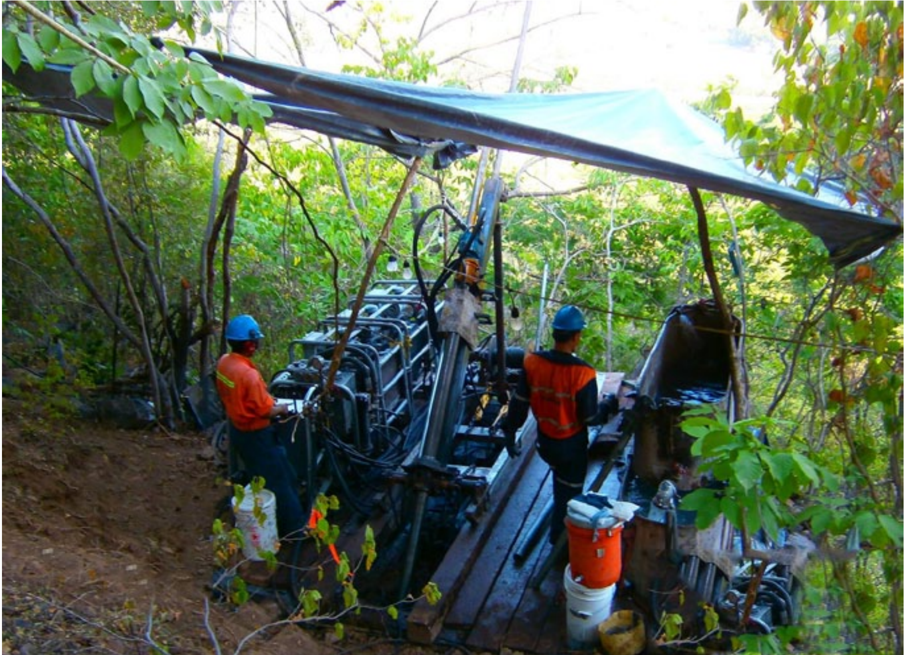
The versatility of our man portable drill rigs allows US Gold to operate on steep hill sides where traditional track or truck mount rigs could not. Picture taken from Palmarito deposit.
