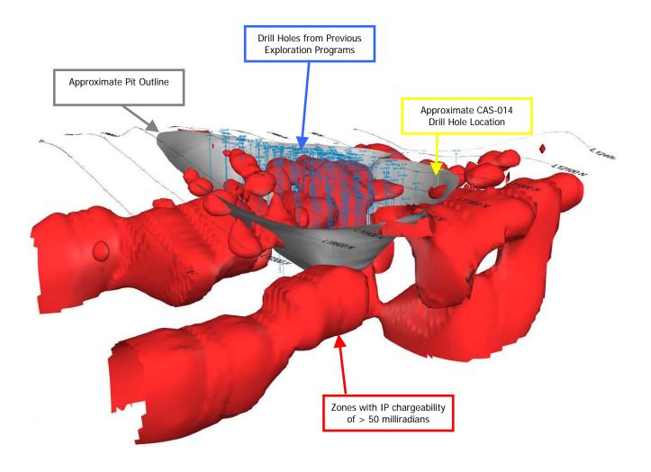
Figure 1: 3-D visualization showing IP chargeability zones (red) in relation to the approximate pit outline and drill holes from previous exploration programs (1969-1971, 1992-1994). Approximate location of new drill hole CAS-014 shown in yellow. IP chargeability zones (red) are isoshells interpolated from vertical 2D inversion sections of IP chargeability along the survey lines.
