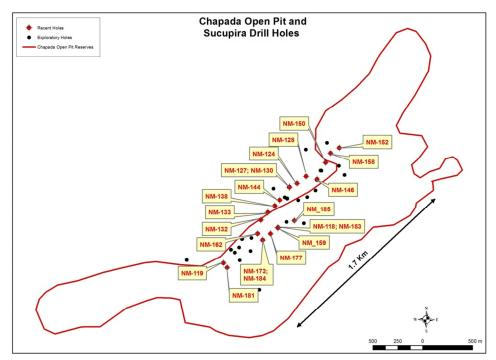
Figure 3: Plan view of the Sucupira drill hole collar locations and the current outline in red of the Chapada Main Pit.
