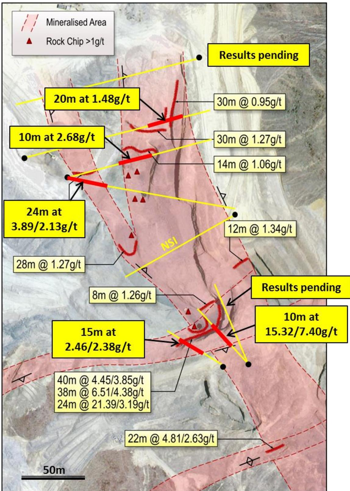
Figure 2: Liseiwi Surface and drill results
