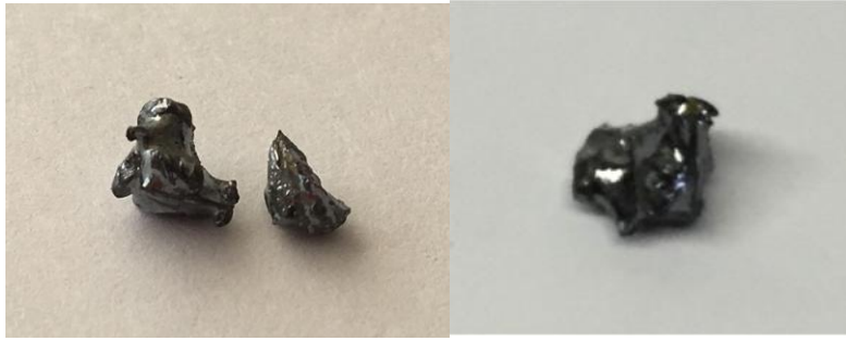
Image 1 – First nuggets of Silicon Metal produced during test #15 (Size about 5x5x8 mm)
