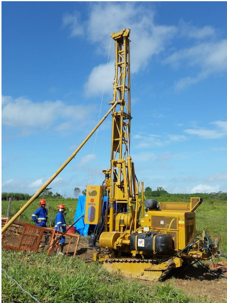
MAC-320 Diamond Core Drill Rig at Jaibaras Diamond Project
